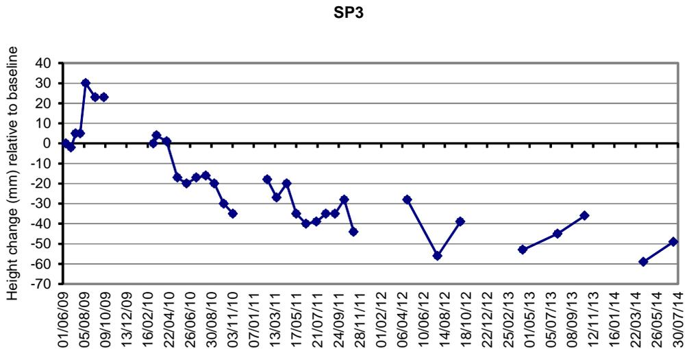
—■ Sediment elevation change (mm) measured at each stake (SP1, SP2, SP3)
