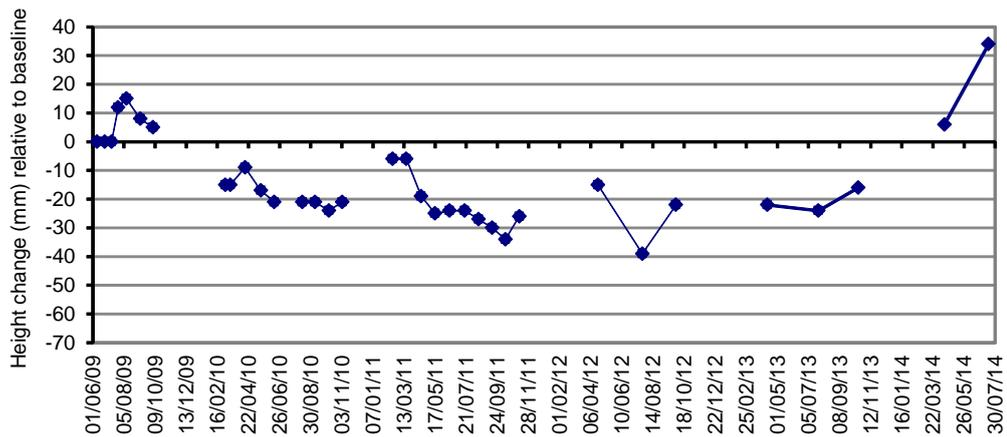
—■ Sediment elevation change (mm) measured at each stake (SP9, SP10)
