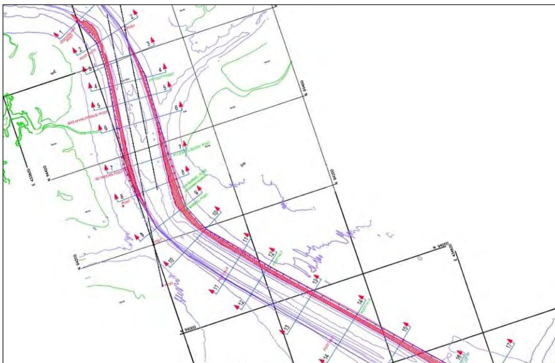
Image 7. Channel margins which LHC propose to dredge to maintain navigable depths
