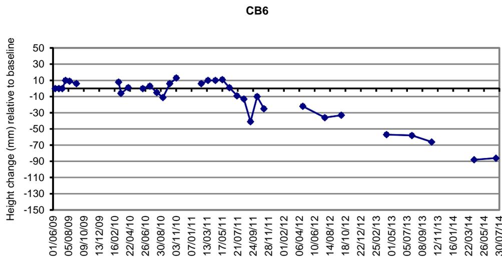
—■ Sediment elevation change (mm) measured at each stake (CB4, CB5, CB6)
