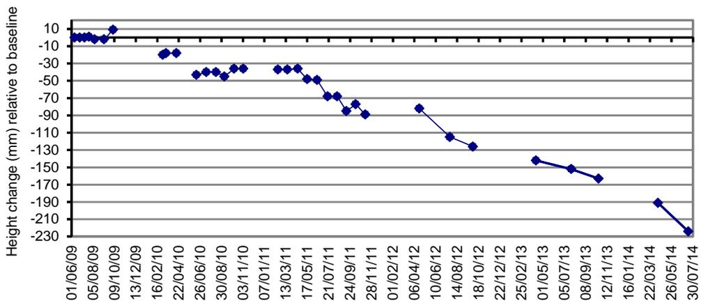
—■ Sediment elevation change (mm) measured at each stake (CB9, CB10)
