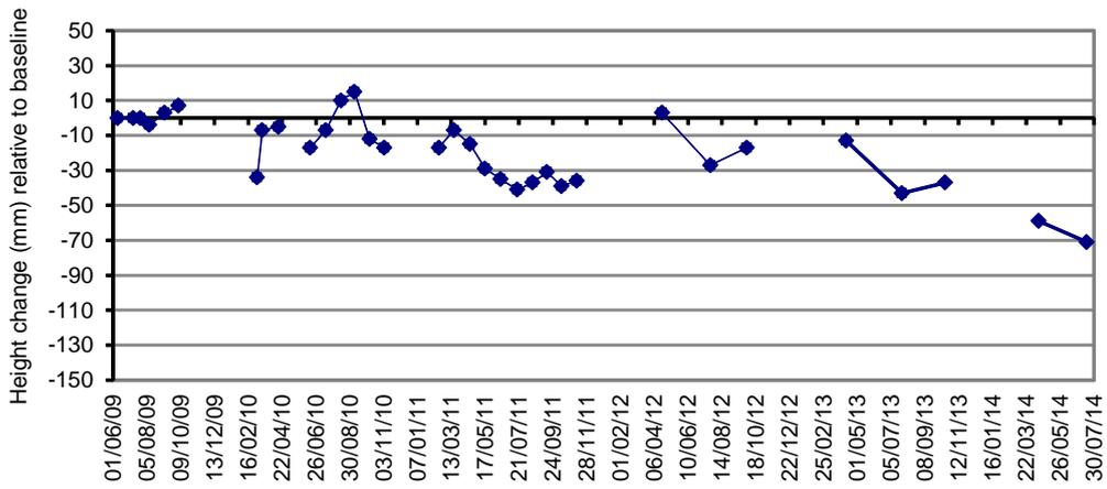
—■ Sediment elevation change (mm) measured at each stake (CB7, CB8)
