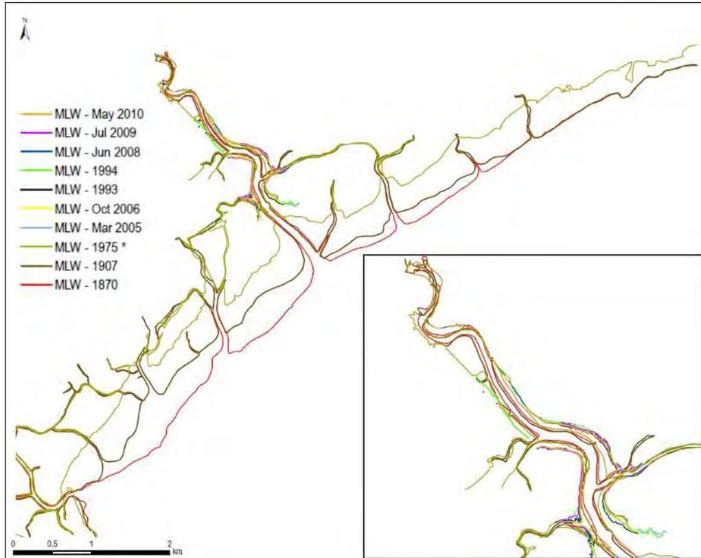
Image 3. Alignment of mean low water showing progressive retreat especially of exposed areas
