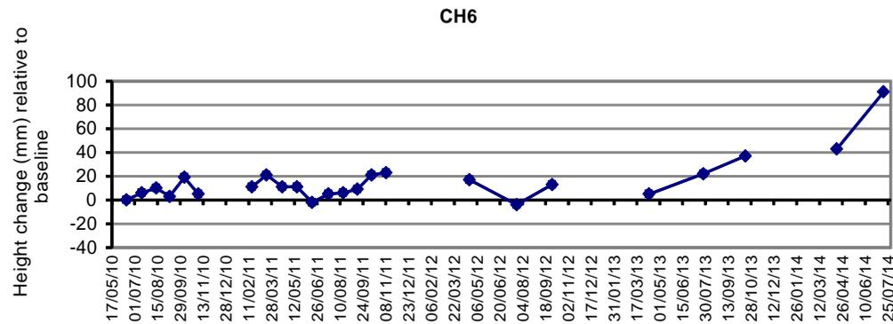
—■ Sediment elevation change (mm) measured at each stake (CH3, CH4, CH5, CH6)
