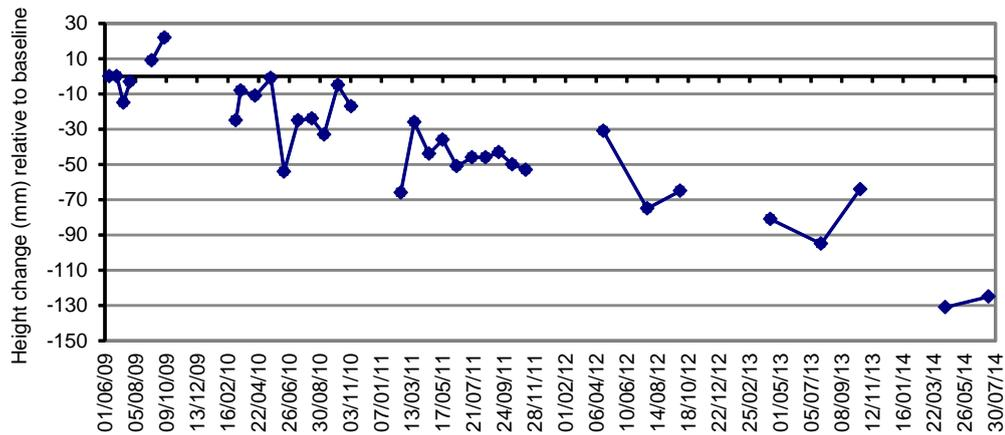
—■ Sediment elevation change (mm) measured at each stake (TB1, TB2)
