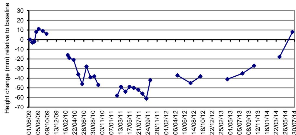
—■ Sediment elevation change (mm) measured at each stake (SP4, SP5, SP6)
