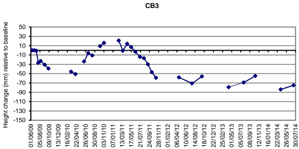
—■ Sediment elevation change (mm) measured at each stake (CB1, CB2, CB3)
