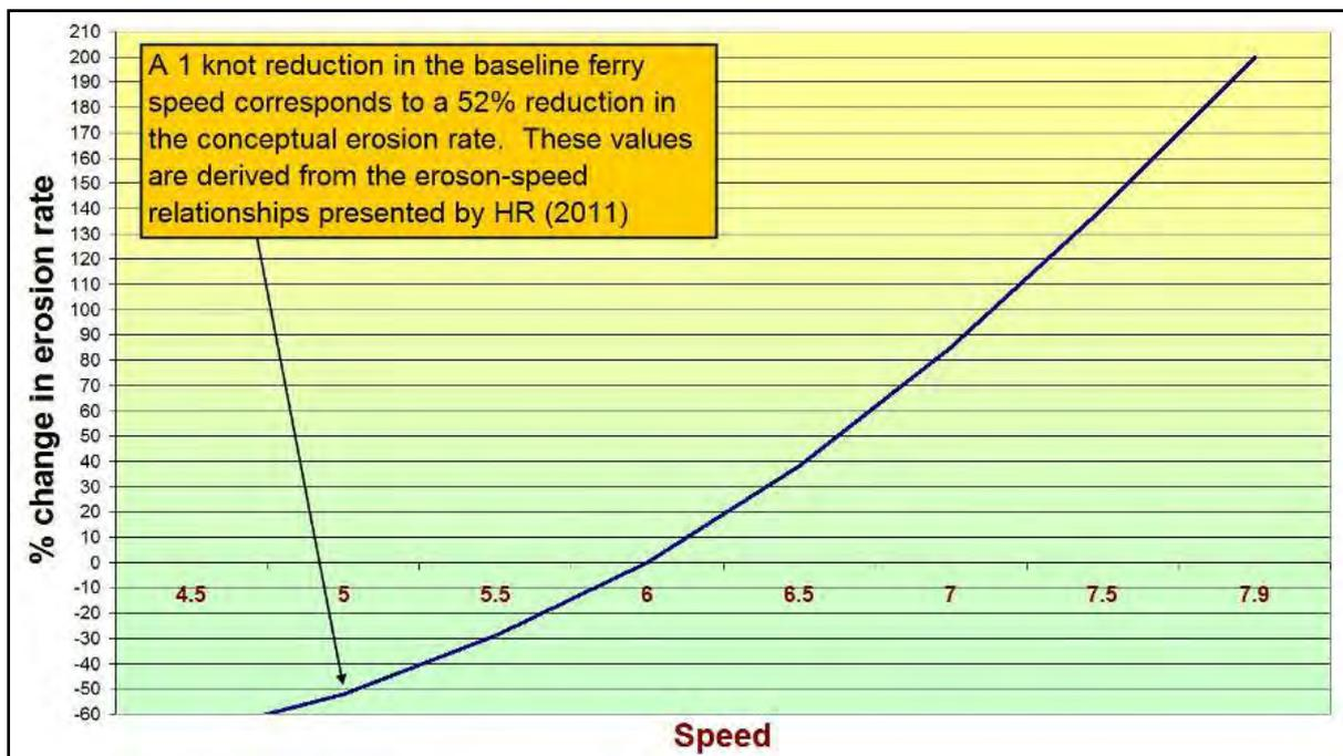
Image B1. Projected relationship between erosion and ferry speed as used within the conceptual impact model
